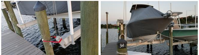
4. Pull drain plugs and check bilge pumps. This will be key with significant rainfall. Your boat can quickly fill up with water and alter its balance on the lift.
